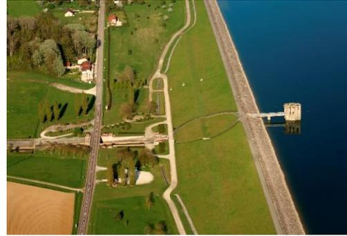
© Photo Chantiers de France porous bituminous facing placement (Radonvilliers dam)
