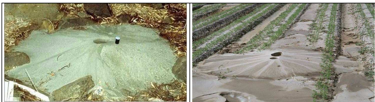
Figure 5-15 - Volcan de sable (sand boil) - craterlet
