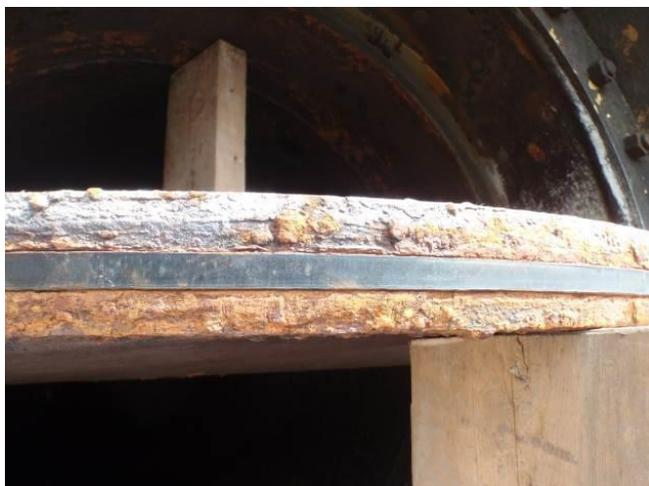
Figure 2.7 – Inspection of the condition of the butterfly valve in a draw off pipe
