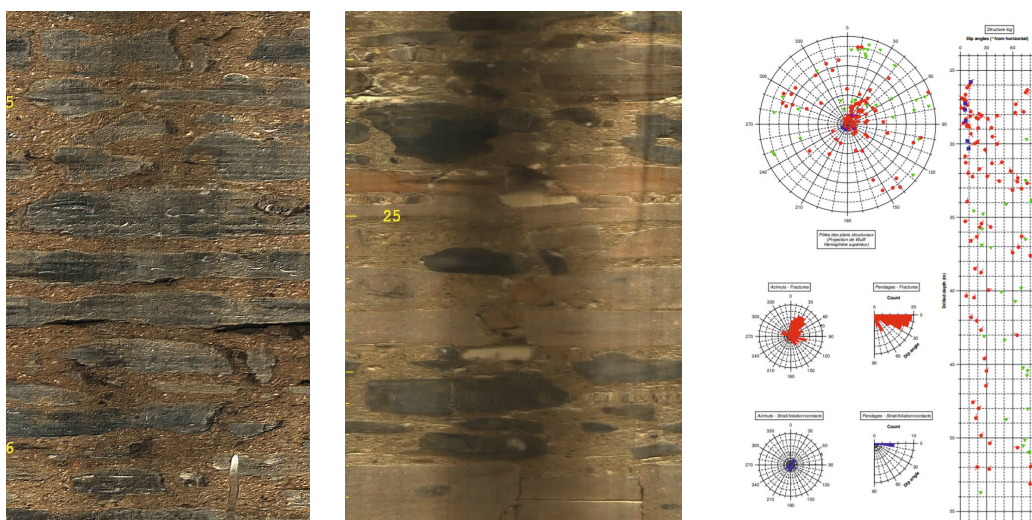
Figure 5.6 – Imaging in drill holes, Pont-et-Massène dam / © Lim Logging
