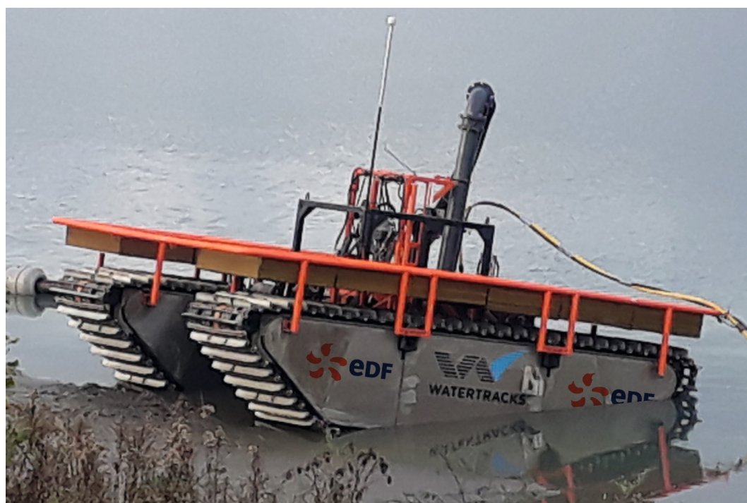
Figure 4.2 – Dredging robot / © EDF
