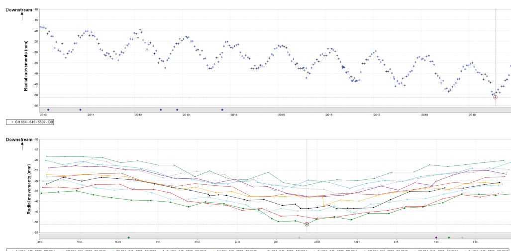
Figure 11.10 – Representation of the radial displacement of the central block of an arch dam affected by an alkali-response pathology: as a function of time (top graph) and over annual periods (bottom graph) / © EDF
