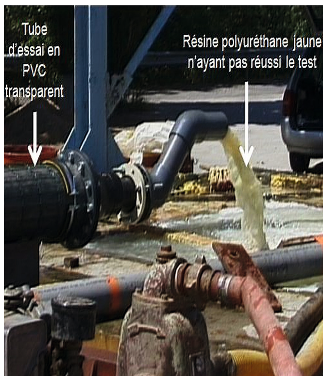
Figure 2.16 – Resin tests at EDF-TEGG laboratory in 1999: turbulent flow through pebbles with water cooled first to 10 °C then to 2 °C through a 10 m long transparent PVC hose / ©EDF
